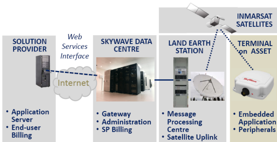
Working System of Satellite Communication Technology
